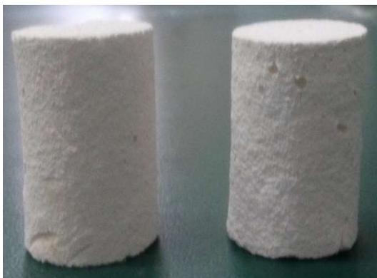
Fig. 2 - Images of the bio-sandstones obtained by mixing process.
