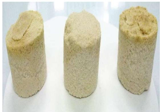
Fig. 4 - Images of the bio-sandstones obtained by bio-grouting process.
