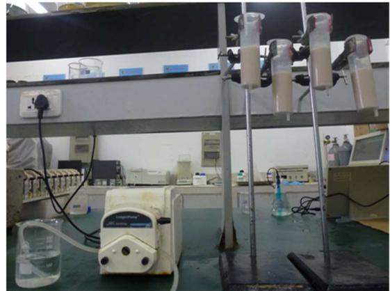
Fig. 3 - Sand column cemented by bio-grouting process.
