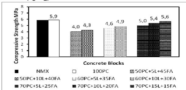
Fig. 3 - Compression strength of concrete blocks cured with steam for specimens reference and ternary system PC – L – FA.
