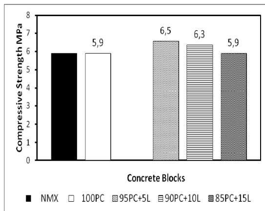
Fig. 2 - Compression strength of concrete blocks cured with steam for specimens reference and binary system PC – L.
