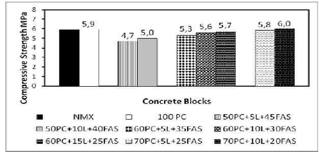
Fig. 4 - Compression strength of concrete blocks cured with steam for specimens reference and ternary system PC – L – FAS.
