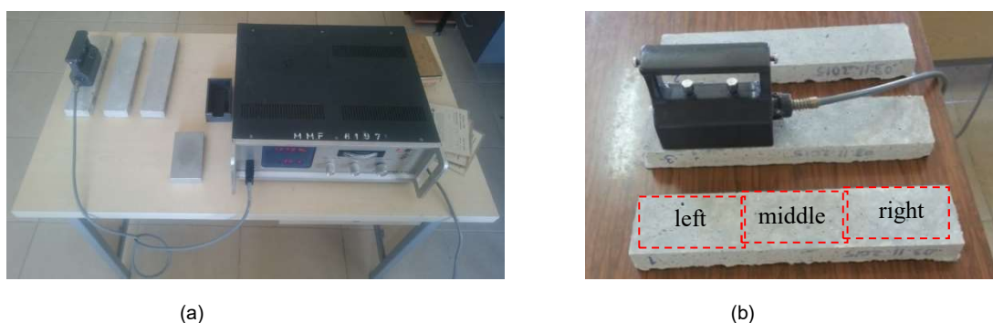
Fig. 5 - a) Thermal conductivity test setup, b) Measurement method.
